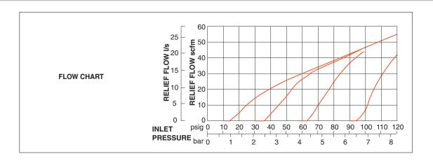
**Relief Valves** have maximum relief flows of 10 to 20 scfm (4.7 to 9.4 l/s). For models with increased sensitivity at lower pressure, consult ROSS.
